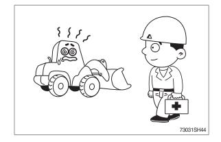
Park on a flat place for inspecting and repairing and properly TAG machine is not operational. (remove start key)
