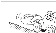
Avoid parking and stopping on a slope. Lower the bucket to the ground and block the tire when parking.
